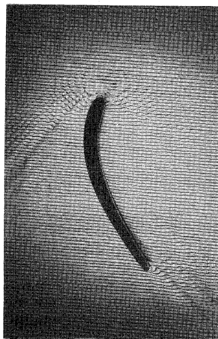
Fig. 3 Cambered airfoil at Mach number 1.86.
